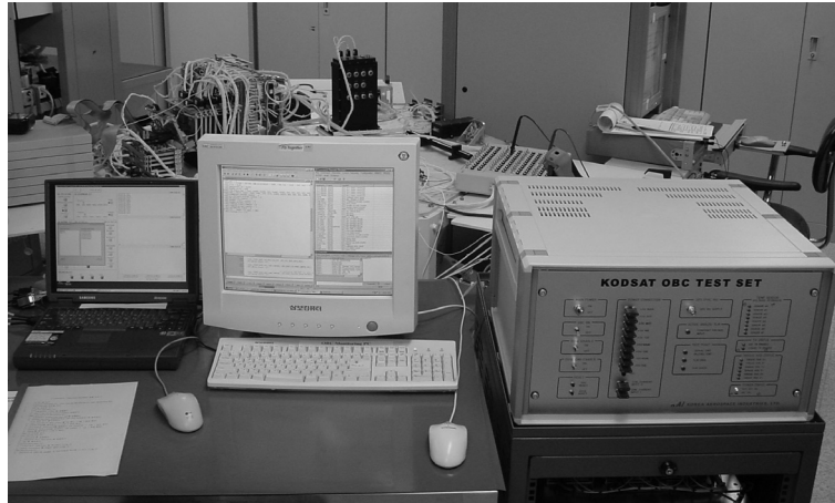
Figure 4. Flight software build test configuration.
